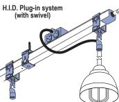
Fixtures, supported by P2855 hangers and M2250 eyelets, plug into receptacle mounted in P2763 outlet box. P2855 hangers also support raceway. P2521-75 end connector joins conduit to raceway. P1280W end caps (not shown) and P3184 closure strip complete assembly.
