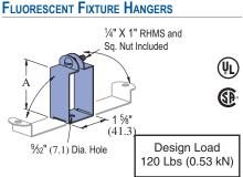
• Hanger provides more than 1/2" (12.7) space between channel and fixtures. Materials: 18 gauge (1.2).
