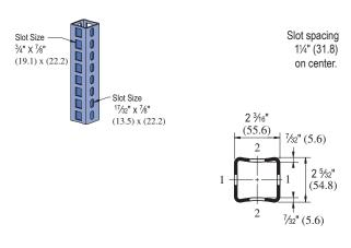
Tubing Finishes: PL, GR, HG, PG; Standard Lengths: 10' & 20'
