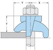
Note 1: When installing, ensure the straight (not tapered) leg of the saddle is in contact with the flange. Note 2: Y, X and T will vary depending on the thickness of V.
