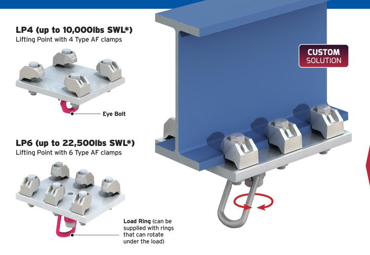
👂 The Type LP can be supplied with either an Eye Bolt or Load Ring. Please state your requirement when ordering.
