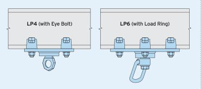
For example, the LP6 has six M24 Type AF clamps to create a Safe Working Load of up to 22,500lbs (4:1 Factor of Safety). Provide details of the loading, rotation, angle and beam dimensions and Lindapter's team of Engineers will design a connection solution to suit your needs.
